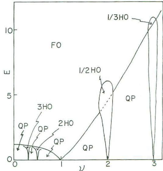
Fig.1. Phase diagram of forced van der Pol oscillator.
